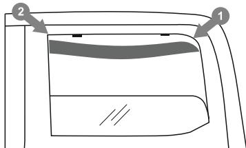
7. The deflector must be installed starting at the back. To do so, place the back part of the deflector frame into the channel and move the front part upwards. Position the entire deflector frame into the window channel, placing the frame between the fastening brackets and the rubber seal as is shown in the picture.
