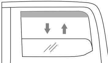
10. Raise the window until it touches the deflector. Carefully pulling the deflector outwards, roll up the window with abrupt movements. Repeat this action 4-5 times, then leave the window closed.
