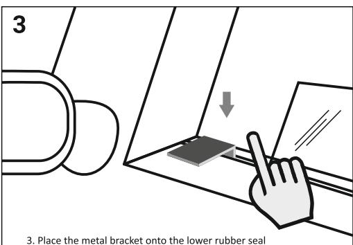
3. Place the metal bracket onto the lower rubber seal as close to the front window frame as possible.
