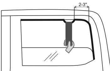
2. To position the fixture, bend the edge of the rubber seal from the back frame of the window by 2-3 inches by using a special metal plate as is shown in the picture.
