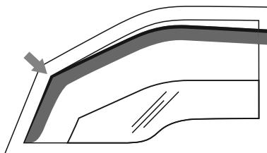
6. Shift the deflector forward, fitting the deflector frame into the channel completely. Make sure the deflector is placed above the lower window frame.
