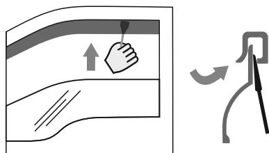
10. To ensure better installation of the deflector and better adhesion between the tape and the surface of the rubber seal, it is strongly recommended that you use the plastic blade, moving it slowly between the window's inner rubber seal and the deflector.
