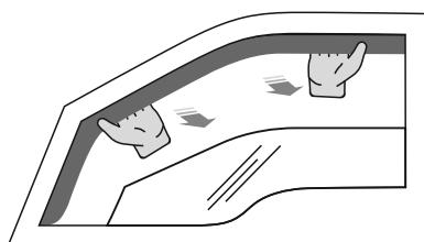
9. Immediately after installing the deflector, adjust its position by carefully pulling it outwards.
