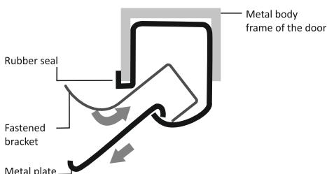
3. Place the fastening bracket in the channel and return the rubber seal to its original position.
