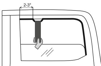
5. Bend the edge of the rubber seal from the front frame of the window by 2-3 inches. Place the fastening bracket in the channel and return the rubber seal to its original position.
