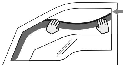
7. Bending the center part of the deflector outwards, insert the back part of the deflector into the channel, leaving a gap above it.
