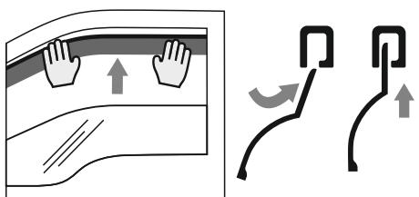
8. Starting with the front part of the deflector, insert it into the window channel.
