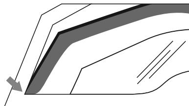
5. Lower the front part of the deflector onto the metal bracket as shown in the picture.
